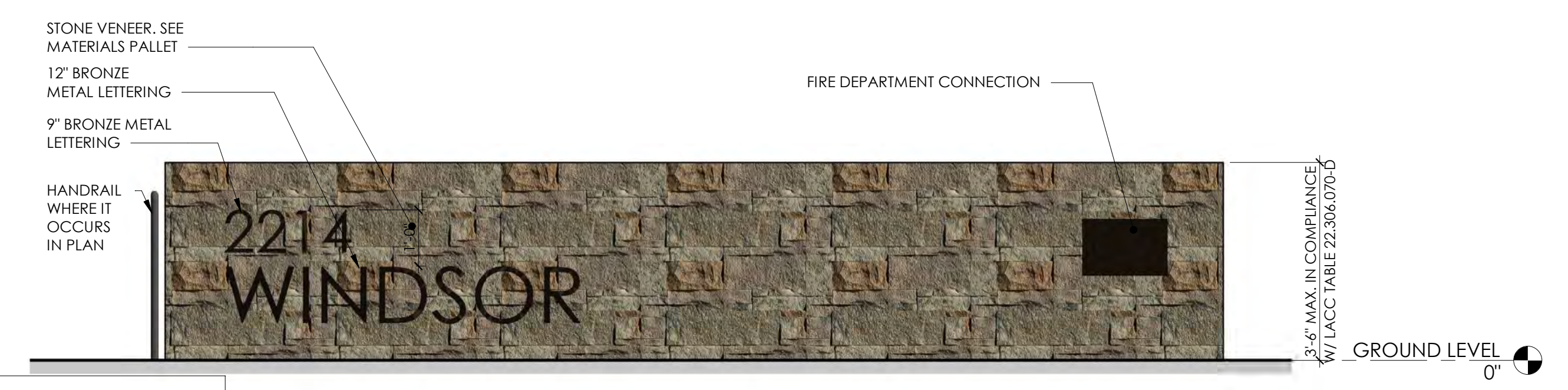
BUILDING IDENTIFICATION SIGNAGE 4 SCALE: 1/2" = 1'-0"
