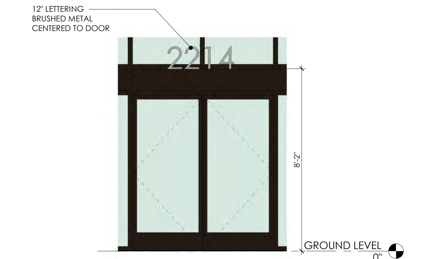
RESIDENTIAL ENTRY SIGNAGE DETAIL 5 SCALE: 3/8" = 1'-0"
