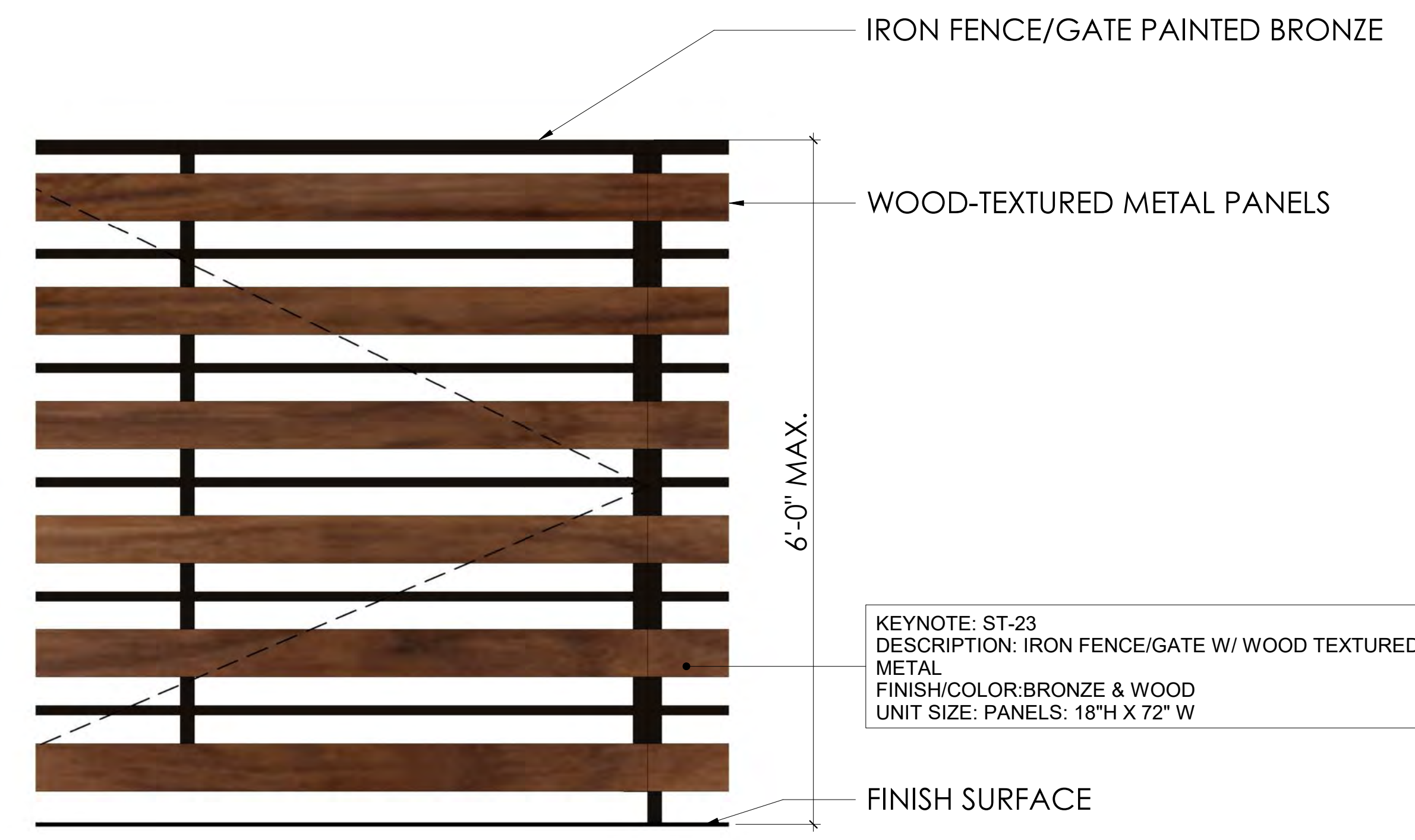
IRON FENCE/GATE DETAIL 2 SCALE: 1" = 1'-0"
