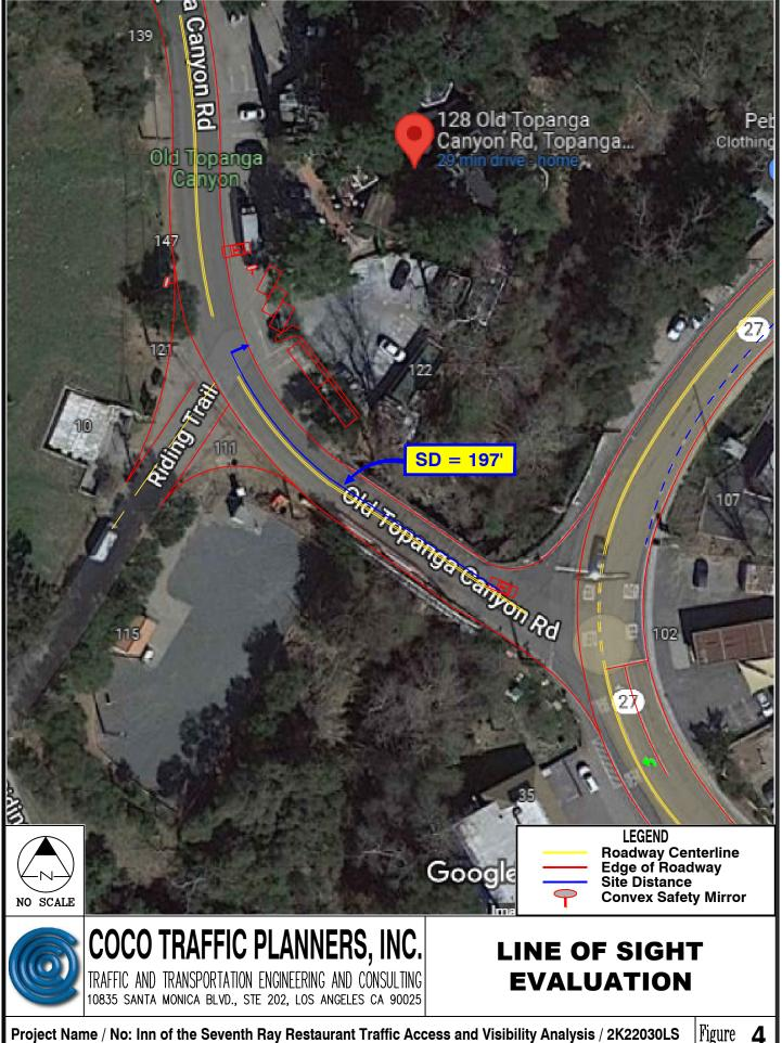
and 200' for eastbound traffic is significantly higher than the minimum required for the observed speeds. At the posted speed limit of 35 mph the required Stopping Sight Distance would be about 186.9'.
