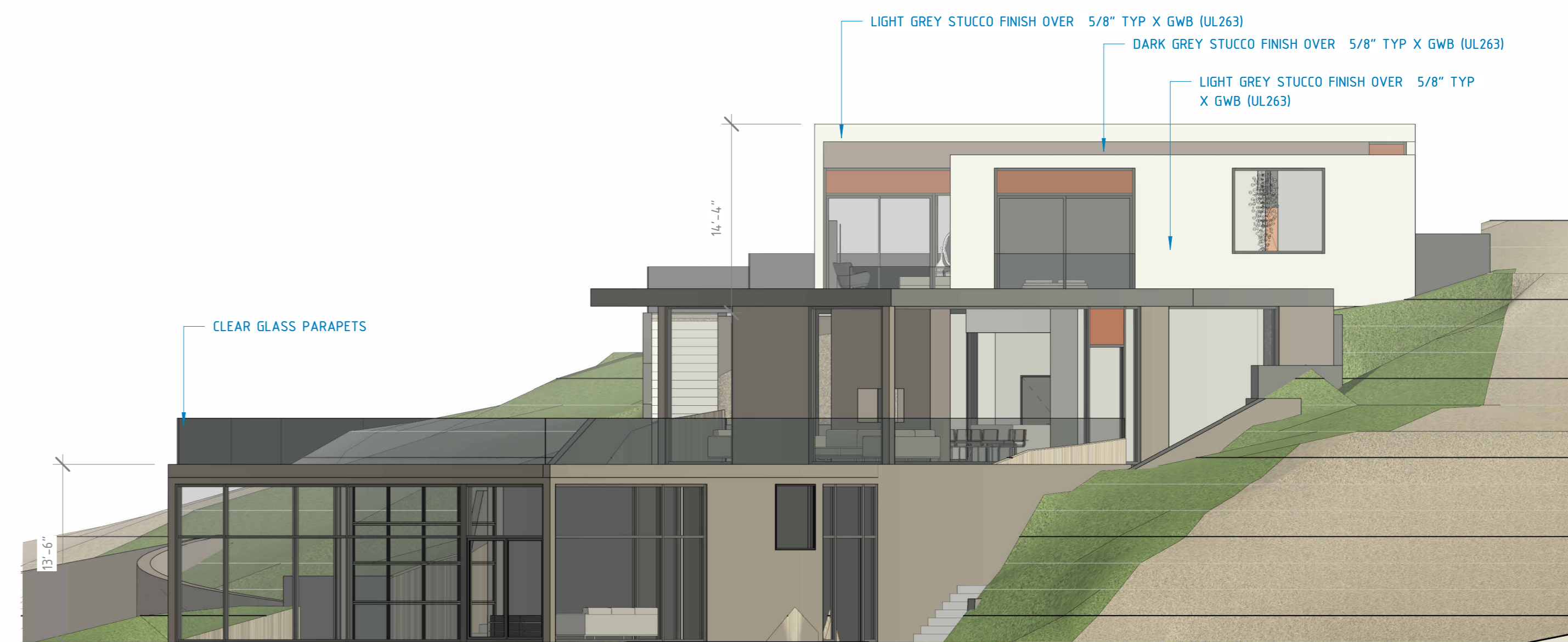
3 WEST ELEVATION (SIDE) 1/8" = 1'-0"
